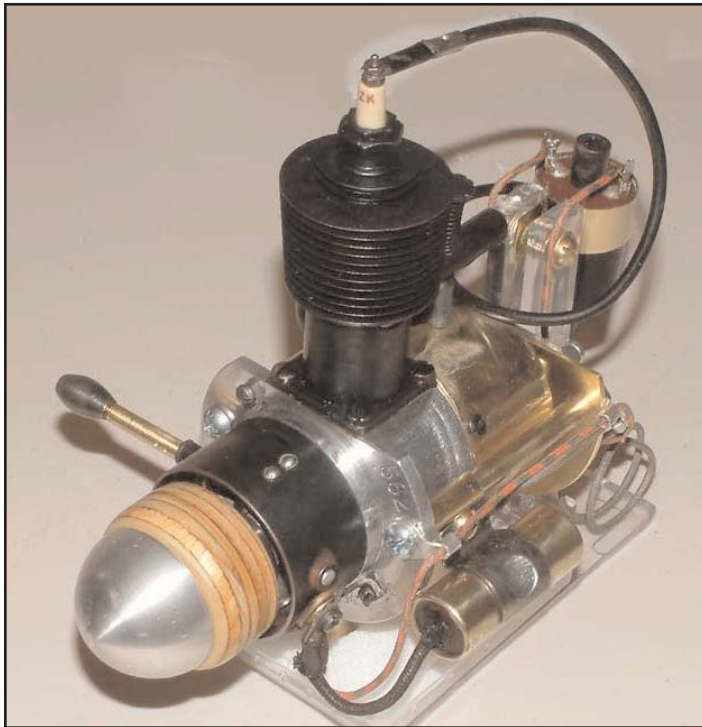
At the forefront of Dennis' display was this Kratmo .57 engine he restored from the rusted relic shown in last month's Flight Lines. In addition to the great restoration job, he added an ignition coil and condenser. More information on this engine is on page 6.
