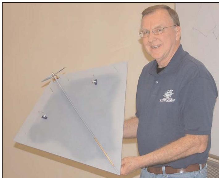
Paul Geders discussed the design concepts and problems encountered in designing and building his delta aircraft made from 6 mm Depron with carbon fiber reinforcement. It has an outrunner motor that is rated at 27,500 rpm, driving a 6-4 prop. Weight is 21.35 ounces.
