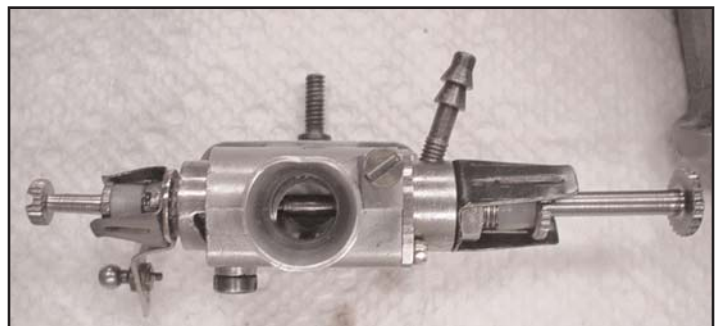
The carb barrel was frozen and had to be heated to disassemble. All parts were cleaned and reassembled, then flow checked.
