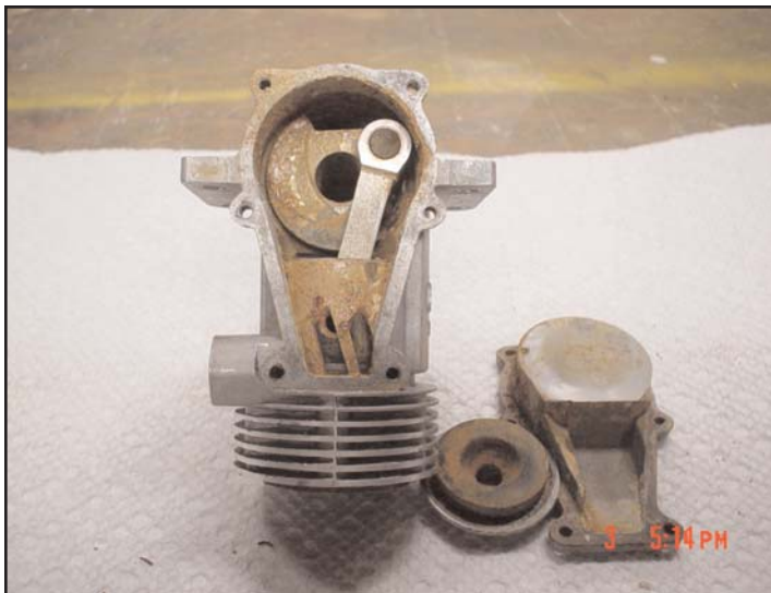
Wow! Notice flakes of rust on paper towel & throughout the crankcase.
