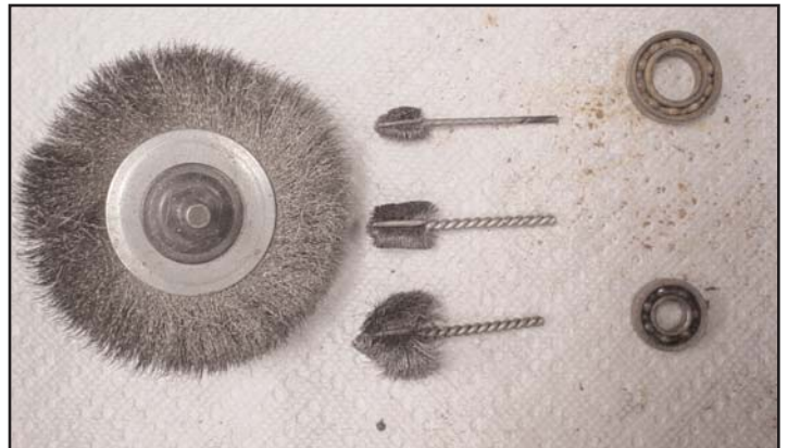
Some of the wire brushes used to clean it up. To get most of the rust off the steel parts, I used a bench grinder with a 7" stiff wire brush wheel. A drill press was used with some of the smaller drill type brushes to clean bore of crankshaft, carburetor barrel, etc.
