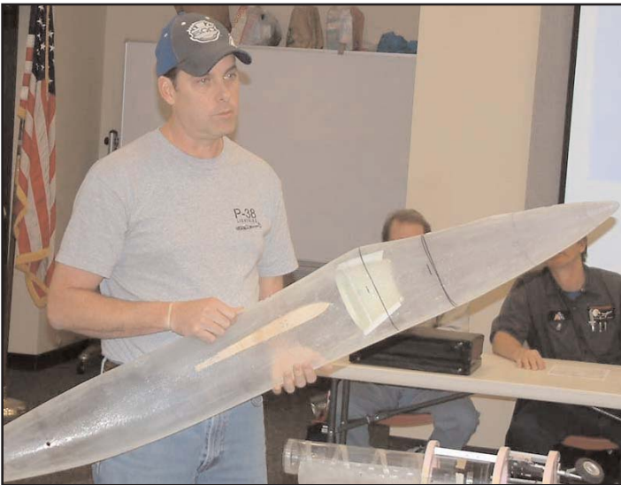
Jeff Bohrer shows the port side of the fiberglass fuselage he designed and formed for his scratch-built Grumman F11F Tiger electric ducted fan jet.
