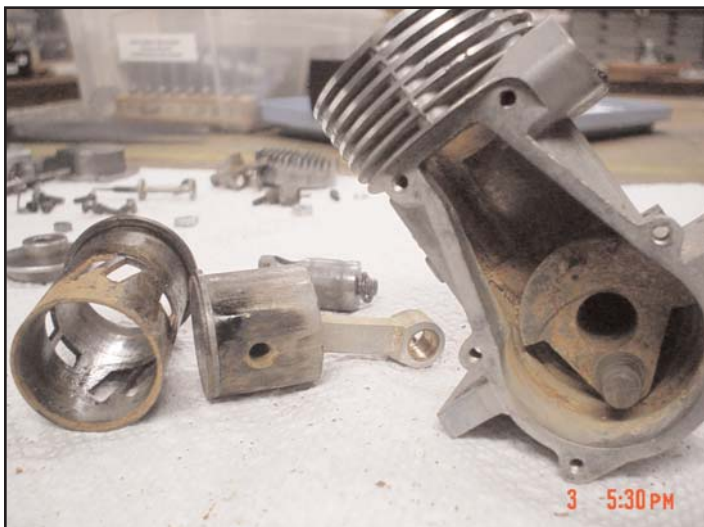
The crankcase had to be heated to get the sleeve out. The piston ring was seized on one side of the piston ring groove.
