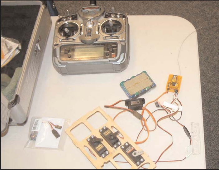
Bob Gizzie's complete radio system with the Orange 9-channel receiver.
