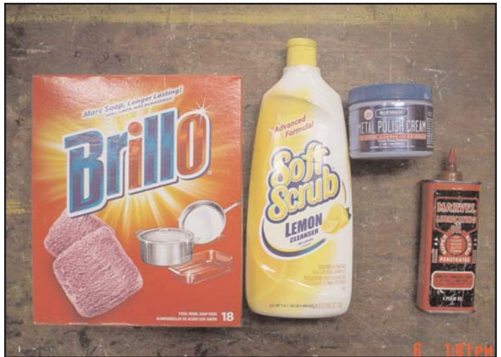
Additional cleaning and polishing materials. Automatic Transmission Fluid is in the Marvel Oil can. Brillo pads are used to polish aluminum initially, followed by Blue Magic Metal Polish Cream. Soft Scrub is used with water and a toothbrush on the outside of the engine before disassembly. I also used a buffing wheel and jewelers rouge
