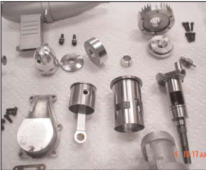
After rust removal and polishing. 600 wet-n-dry sandpaper with ATF was used to polish the sleeve inside and out, and the crankshaft. I used a 3" cloth buffing wheel and jewelers rouge on both steel and aluminum parts.
