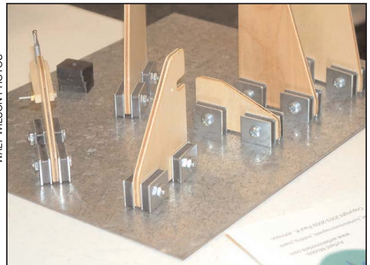
The magnets are attached to the plywood clamps with standard screws and nuts. His entire building board is covered with a sheet of galvanized steel. Pins are no longer used to hold parts in place in his workshop! Parts and building information are available at: http://www.airfieldmodels.com
