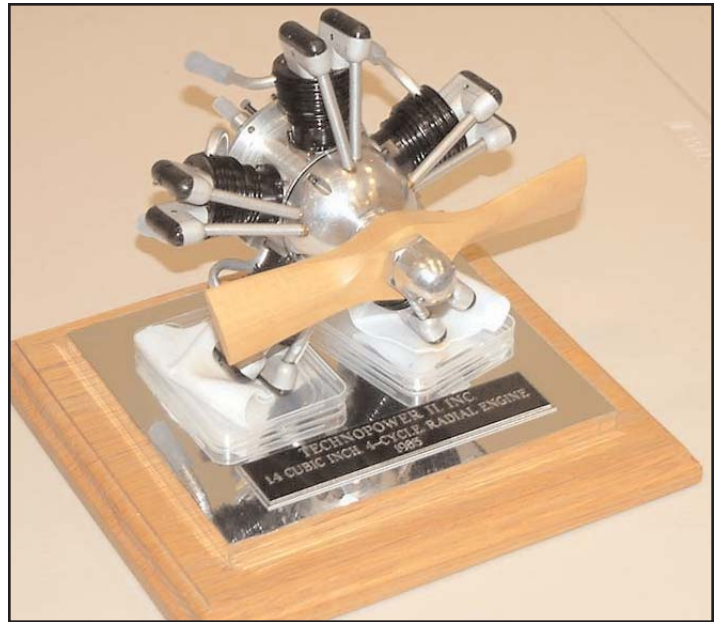
Dennis also displayed this Technopower five-cylinder radial engine. After purchasing it, he completely disassembled and cleaned it up. He has run it and says lighting five glow plugs at the same time is really fun!
