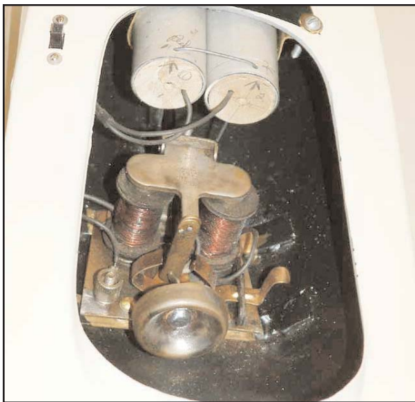
The vibrator motor is powered by four "C" batteries and starts by spinning the flywheel.
