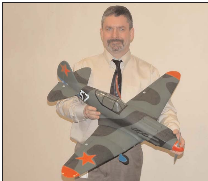
Chris Nenzel discussed this Hobbycity Online Mig 3 ARF. It has a fiberglass fuselage with built-up balsa wings and tail surfaces. He has a 36-30-1400 outrunner motor with a 60 amp ESC and two 2100mAh batteries. Weight is a bit over three pounds and it has a tendency to be touchy to turn or when landing..
