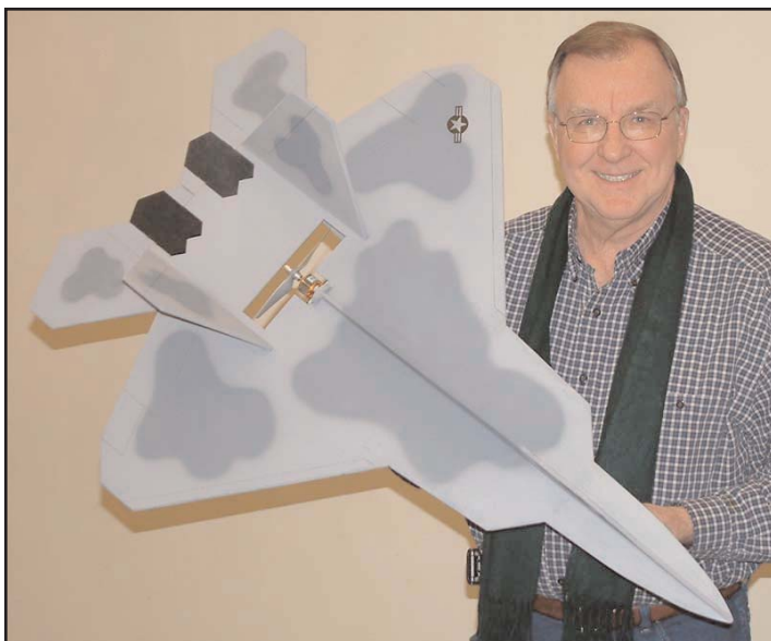
Paul Geders built this profile F-22 from published plans. It's made from 6 MM Depron and features vectored thrust, enabling it to turn in a very small radius. It has been flown and performs very well.
