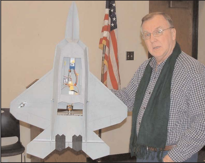
Paul shows the spacious radio compartment in his pro-op driven F-22. The wing has a single carbon fiber spar.
