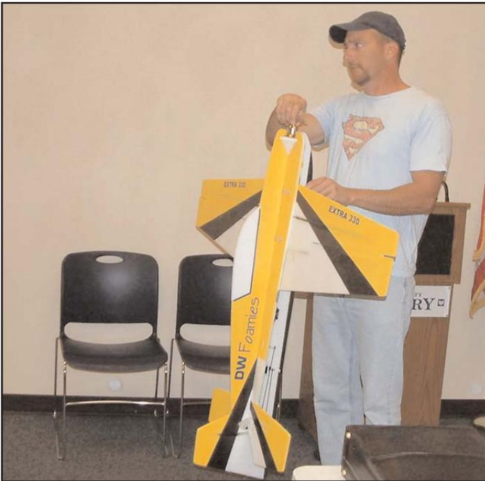
*Tom Foster showed his DW Foamies, Extra 330, large size outdoor, 9 mm Depron foamy with a 1000KV motor and 30 Amp ESC. It weighs 26 ounces and should fly very nicely when the weather stabilizes somewhat.*
