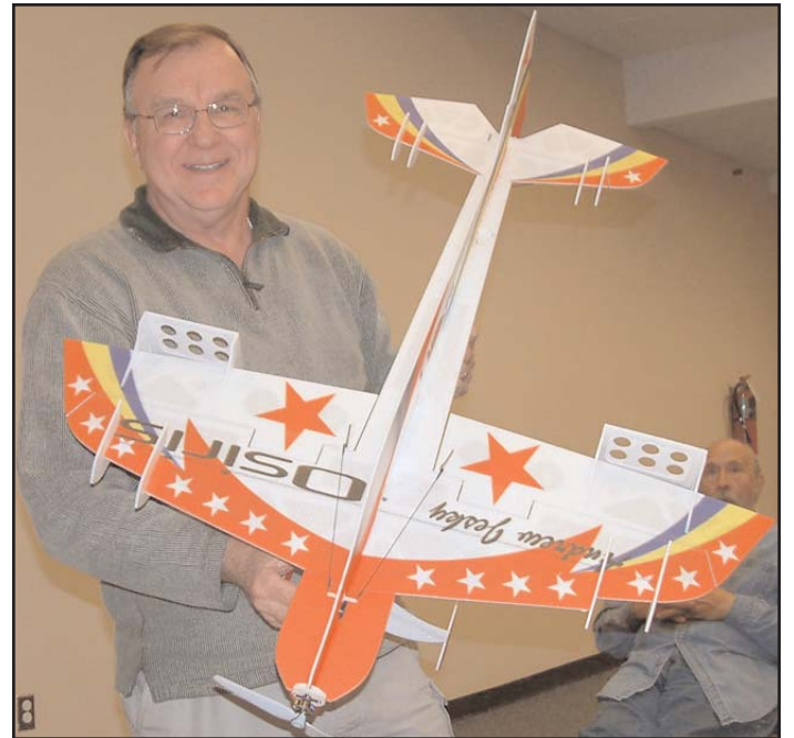
Paul Geders discusses his 4-1/2 ounce. Andrew Jesky Osiris by Fancy Foam that is flown in F3P indoor pattern. The air brakes move with the ailerons for very slow flight and hovering.
