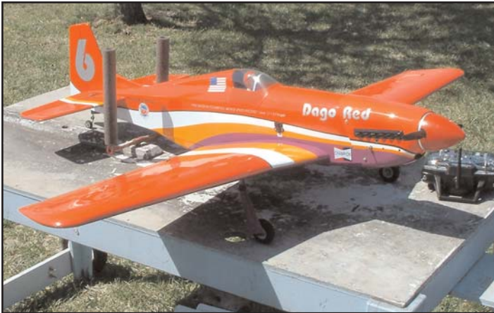
Paul Geders' Dago Red P-51 has a Jett .50 up front and is very fast. He says it also handles beautifully.
