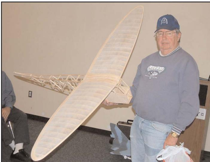
Babe Raab started building this replica of a 1938 Comet Clipper Mark VI 18 years ago. The wing was covered with "silkspan" then and is still tight. He intends to use electric power when it's finished.
