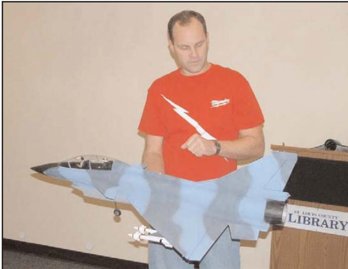
Greg Bohrer showed his GWS Chinese J-10 ducted fan ARF. It comes with a fan, but no electric's. He covered it with heavy silkspan, applied with thinned Titebond glue, and finished it with acrylic paints.
