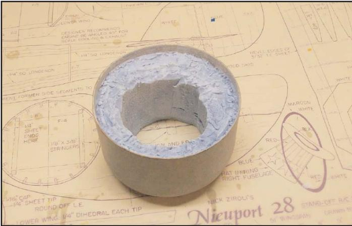
The foam form is shown inside the laid-up fiberglass cowl. The foam can be dissolved or cut away after the heavy-duty cutting and sanding are completed.
