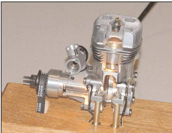
Dennis Skeeters' cut away part of a Super Tigre .61. It's electric powered and has a light to aid viewing while it's being run.
