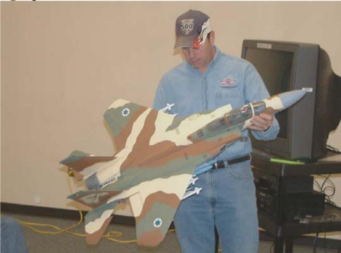
*Jeff Bohrer shows his completed F-15. It's constructed of foam covered with silkspan and wood glue. It has a pusher motor that turns about 27,000 RPM. Jeff designed it around an available manufactured canopy.*
