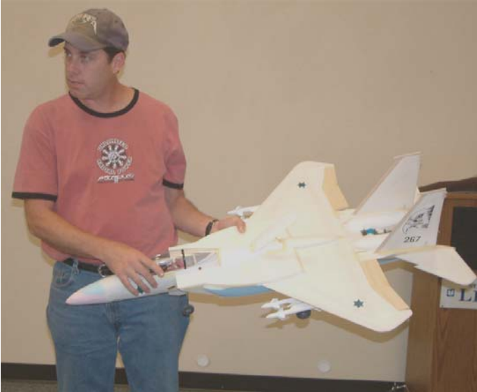
Jeff Bohrer shows his new F-15. It has electric power and is constructed of foam with carbon fiber reinforcements in critical areas. It has a pusher motor that turns about 40,000 RPM! Very nice job! WALT WILSON PHOTO
