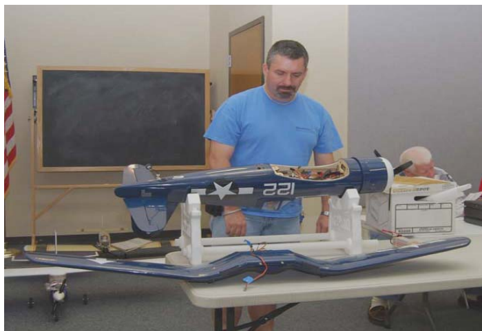
Chris Nenzel discussed his new H&M Performance Corsair ARF. Its electric powered and has retracts. The rotating retracts were troublesome to set up and have caused problems in use. It weighs 8 pounds and has a 600KV Scorpio brushless motor with a 6-cell, 5000 mAh LiPo battery
