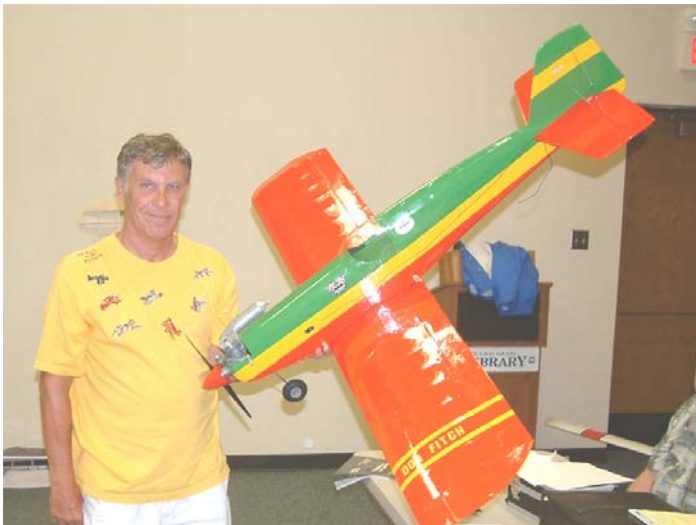
Bob Fiely built this Andrews Sport Master for Don Fitch. It has a Clarence Lee K&B .61 up front and is covered with Monokote. Walt Wilson Photo
