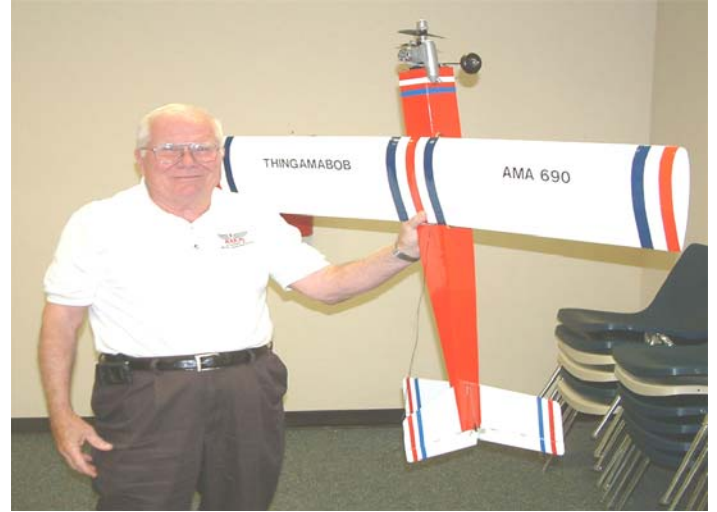
Bob Underwood discussed the 20-year-old "Thingamabob" he designed and built. It was featured, with plans, in a 1990 issue of Model Aviation magazine and is capable of being flown Radio Controlled, Control Line, or Tethered Radio Controlled. A Tethered R/C plane is attached to a center pole with a Control Line wire, then the throttle and elevator are Radio Controlled, for flying. He says it really works! It can also be easily converted to electric power
