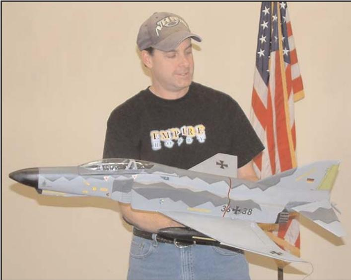
*Jeff Bohrer holds his scratch-built McDonnell F-4. It's constructed of foam board and "pink foam", with carbon fiber rod reinforcement. It has a pusher electric motor and weighs 28 ounces, ready to fly. The little bird flies well, and has been crashed into a tree with minimal damage.*
