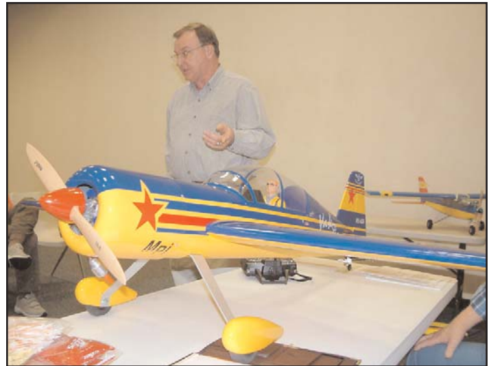
Paul Geders brought his Seagull Yak 54 ARF. It has a YS 1.20 pumper four-stroke up front and will hover at 1/3 power. He used all supplied hardware and a Futaba 2.4 GHz radio with digital servos. He says it's well-built and a great value for the money.
