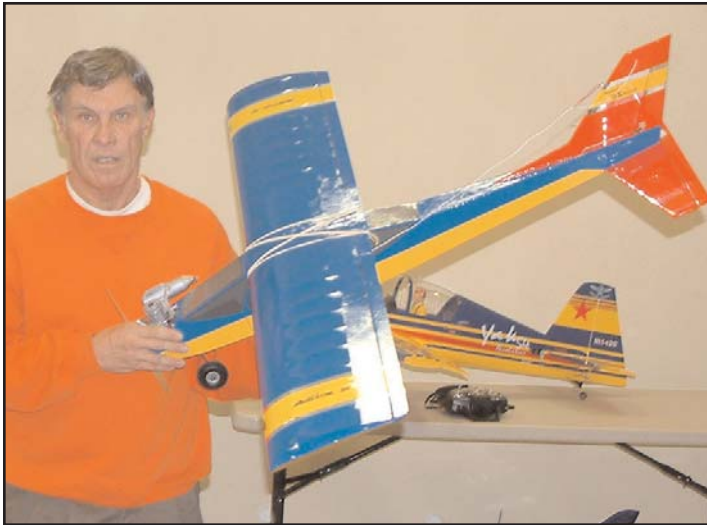
Bob Fiely discussed his Midwest Aerostar 20, built from a kit. It's powered by an O.S. .25 FX. Bob, who likes to build, lamented the fact that so few BIY kits are available for engines in this size range.
