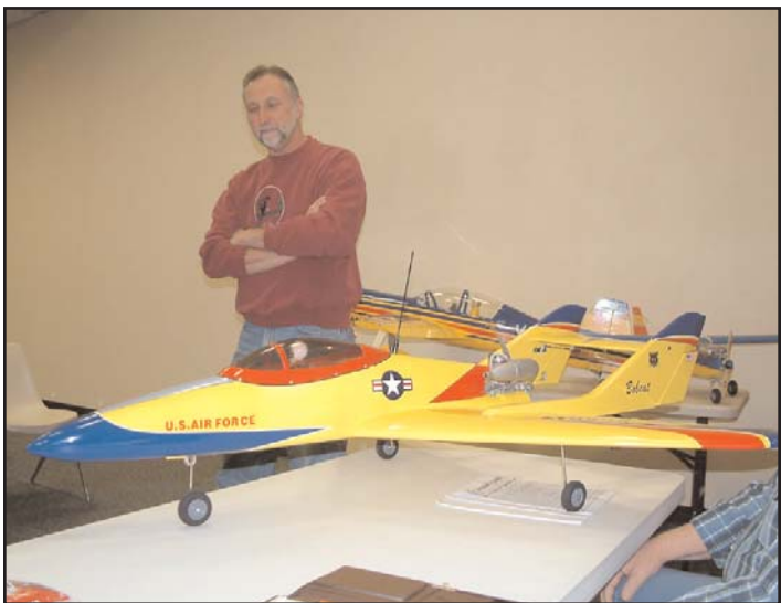
Bill Lindewirth discussed his Nitro Models Bobcat ARF pusher. It has fixed landing gear and an O.S. .61 FX for power. Bill says the hardware and instructions are "junk" and should be discarded. He also had several problems with the layout of servos and other components. The plane is nicely finished and looks good.
