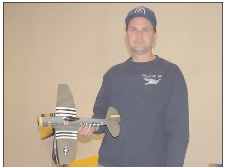
Greg Bohrer gave a presentation on Cox Warbirds with the emphasis on batteries. The P-47 Thunderbolt he's holding has been re-painted and modified to use ailerons, rather than rudder. It's powered by a brushless motor with a LiPo battery. Races this year are planned for both stock and modified classes of Cox Warbirds.
