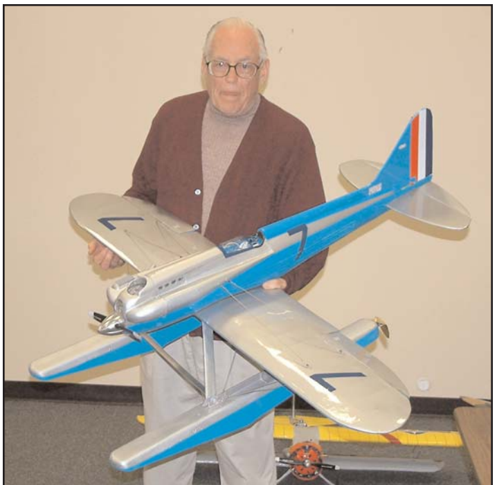
Bill Hancock built this Supermarine S-5 Schneider Cup Racer from scaled-up R/C Modeler plans. In 1931, the full-scale S-5 was the fastest airplane in the world at 404 MPH. The model has Gee Bee foam floats and is powered by an O.S. .46 FX. He overcame several design problems and is looking forward to the Wright Flyers' Float Fly at Innsbrook on Memorial Day weekend.
