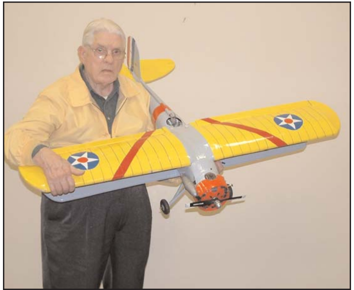
Claud Wade shows his scratch-built Curtiss F9C-2 parasite fighter. It was designed to be suspended from the bottom of the U.S.N. Airship Macon and used for it's defense, in the event of attack. While the aircraft flew well, the concept was soon abandoned. Claud's model is powered by a Fox .50.
