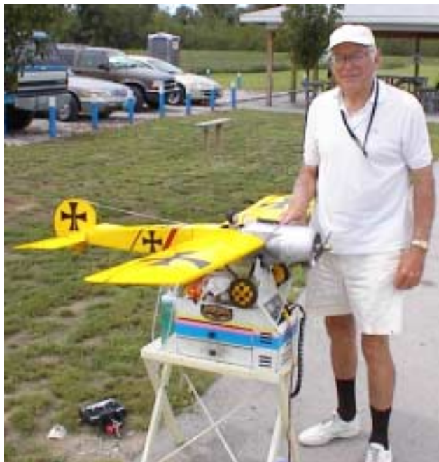
Bill Hancock with his Great Planes Fokker Eindecker. It has a Magnum .52 four-stroke and flies very well.
