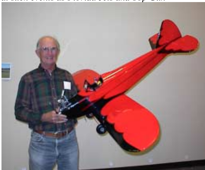
George Cooper shows his Bowers Flybaby. He built it from RCM plans and a pile of lumber. It's powered by a Saito .91 four-stroke and is covered with Ultrakote. It's been flown since the meeting and flies great!
