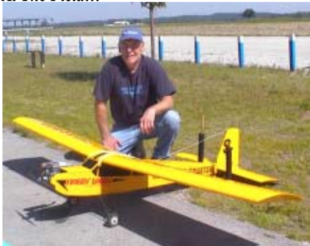
James Frederick with his Senior Telemaster. It's powered by a Super Tigre .90 and flies very well.
