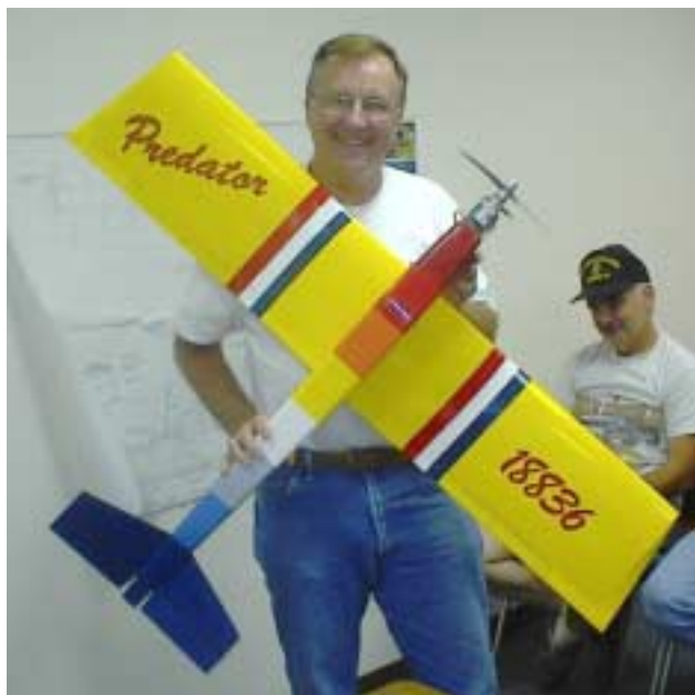
Paul Geders discussed his scratch-built "Predator". He designed it about three years ago to show all the ways flyers could deviate from the intent of the racing rules existing at that time. It has the wheels buried in inverted gull wings along with several other trick features. It turned 134 mph with a Rossi .40 at that time. Now it's powered by an O.S. .25 VF DF for sport flying.
