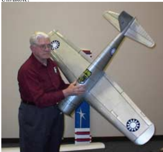
Claud Wade holds his scratch-built Vultee P-66 Vanguard. It's powered by a Fox .50 and is covered with Monokote.
