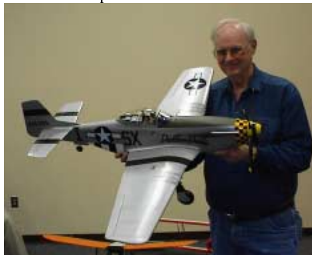
Walt Wilson hold his House of balsa P-51D. He started building it, for Warbirds competition, 16 years ago and still hasn't completely finished it. It has a K&B .40 pumper for power and is finished in Hobby Poxly Aluminum paint over fiberglass.
