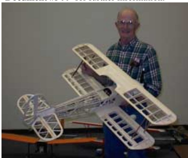
George Cooper was ready to cover his Sig Smith Mini-Bipe, but decided to show his handiwork on the structure. It's a scale model of a plane owned by a friend of his. It has Saito .56 four stroke power.
