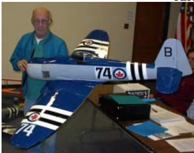
Bob Bennett brought his Top Flite Hawker Sea Fury. It's powered by an O.S. 1.20 FS four stroke engine and has retracts. He had a flywheel made to add weight to the nose. It's finished with Monokote.
