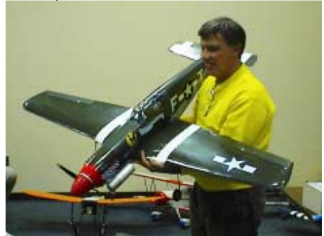
Bob Fiely holds his Top flite P-51B. It has a Super Tigre .61, Hobbico mechanical retracts and is covered with Monokote.
