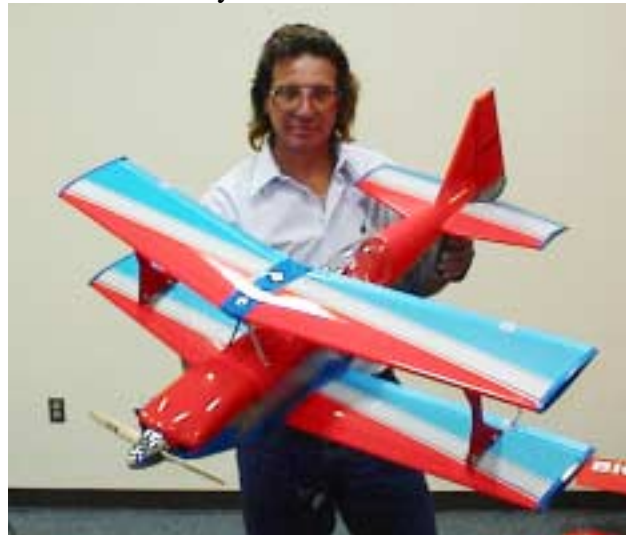
Steve Ramonczuk shows his Kyosho Ultimate Bipe ARF. It's powered by an O.S. .70 FS. As is his practice, he replaced all metric hardware with American equivalents. He had not flown it at meeting time.
