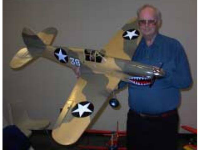
Walt Wilson holds his Kyosho P-40 Warhawk ARF. It's powered by an O.S. .46 FX and has Hobbico 90° rotating retracts. It's a kit review for R/C Modeler magazine and was still in work at meeting time.
