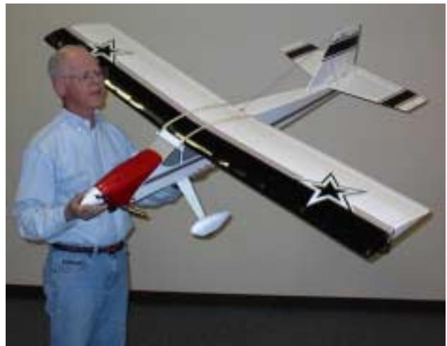
Russ Watts discusses his modified Sig LT-40. It was built from a kit, it's not an ARF. It has a Saito .56 four stroke for power.
