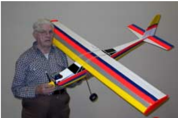
Claud Wade with his scratch-built trainer. It has an O.S. .40 LA engine and flies very well.
