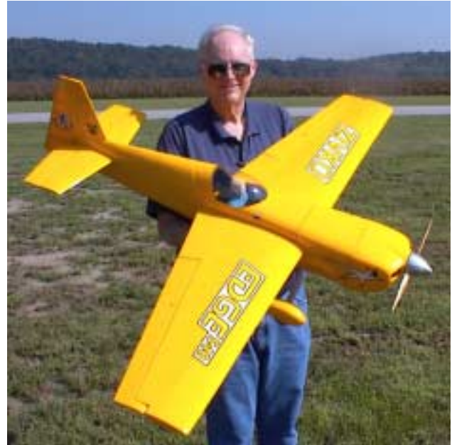
Walt Wilson with his D&L Designs Zivko Edge 540. It's Monokote covered and powered by an O.S. .61 FX.
