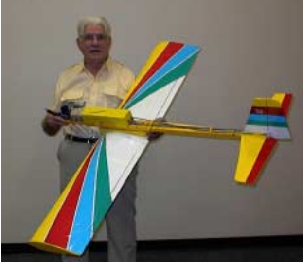
Claud Wade shows his scratch-built test bed for radio components, first flight of the year, etc. It's powered by an O.S. .40 LA and hadn't been flown as of meeting night.
