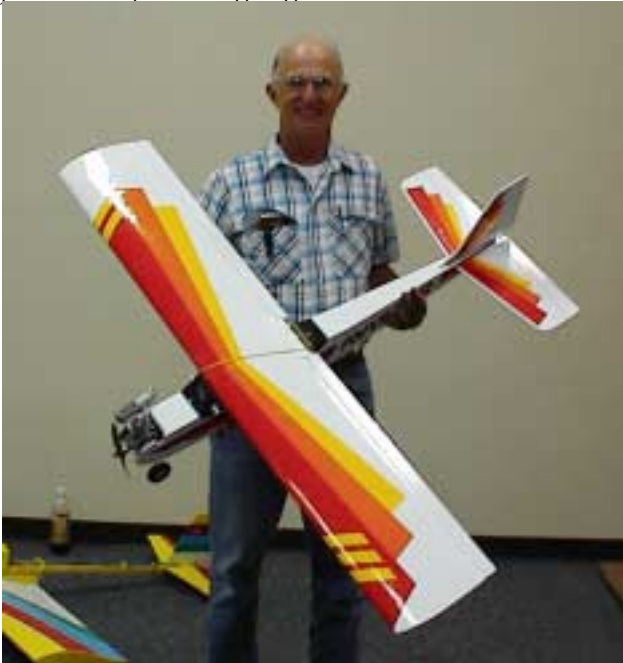
George Cooper holds the rebuilt Avistar club trainer. A number of members contributed parts or money toward it's recovery. It's powered by an O.S. .40 FP and, I'm assured, has more rubber bands on it when flown.
