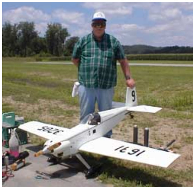
Gene Jones displays his G-Shark ARC. It's built in Mexico and powered by a German Wankel displacing 2.2 cubic inches and spinning a 20-8-14 prop. Weight is 25 to 30 pounds.
