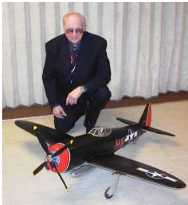
Walt Wilson showed his P-47 M. It's built from a 1/8-scale Top Flite kit. It's powered by an O.S. 1.20 FS engine has Robart pneumatic retracts and operating flaps. The radio is a Futaba 6XA with seven servos.
