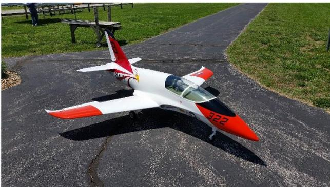
I am using an older, original Titan from *Jetcat*. Propane start. Rated at 36lbs thrust from the manufacturer but I have a feeling it isn't developing quite that much.
