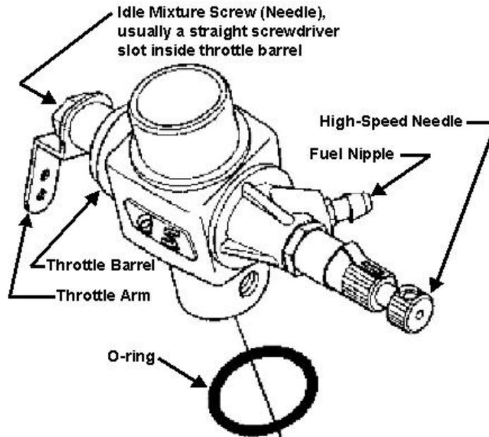
**This is a typical “2 needle” carburetor without a “throttle stop screw”.**
